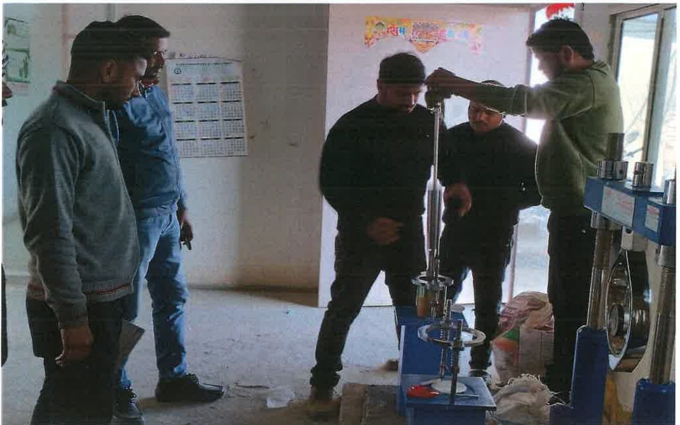
DBM Mould Casting for DBM Mix Design Under Process.
