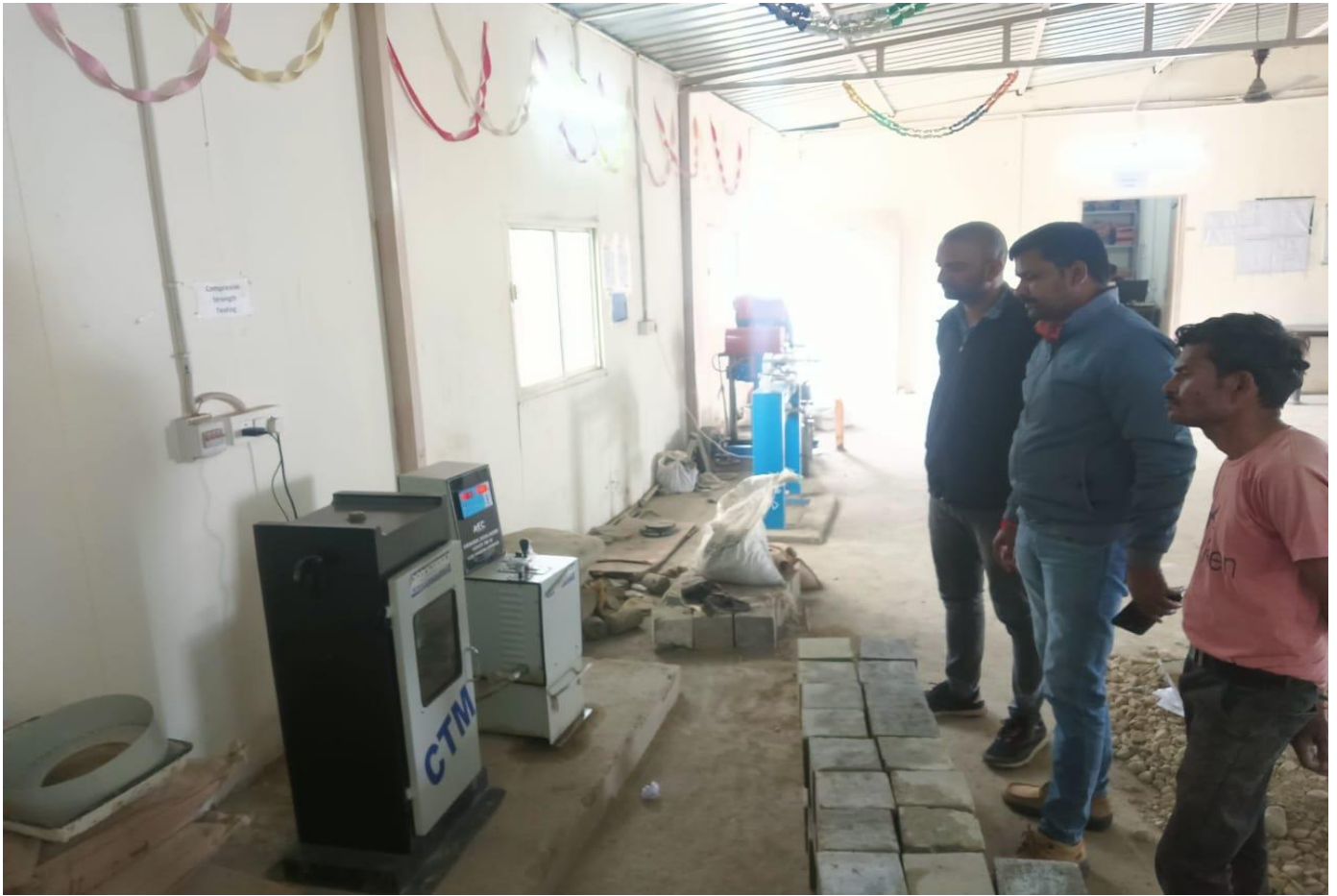
Concrete Cube Testing going on with AQME sir
