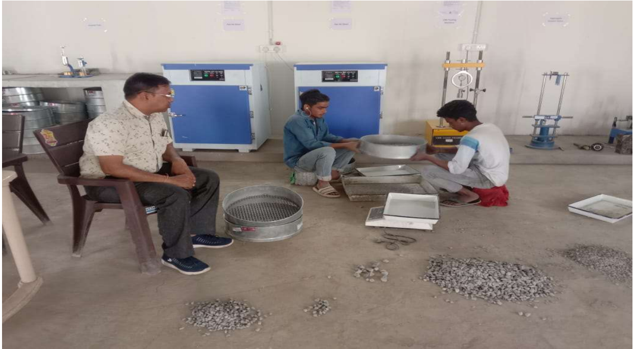
Gradation of Coarse Aggregate
