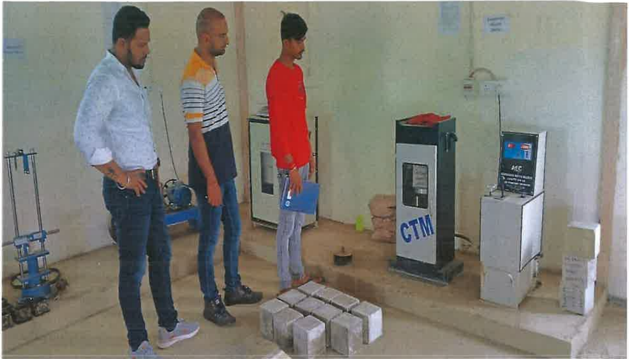
Concrete Cube Compressive Strength Test in Presence of IE Team
