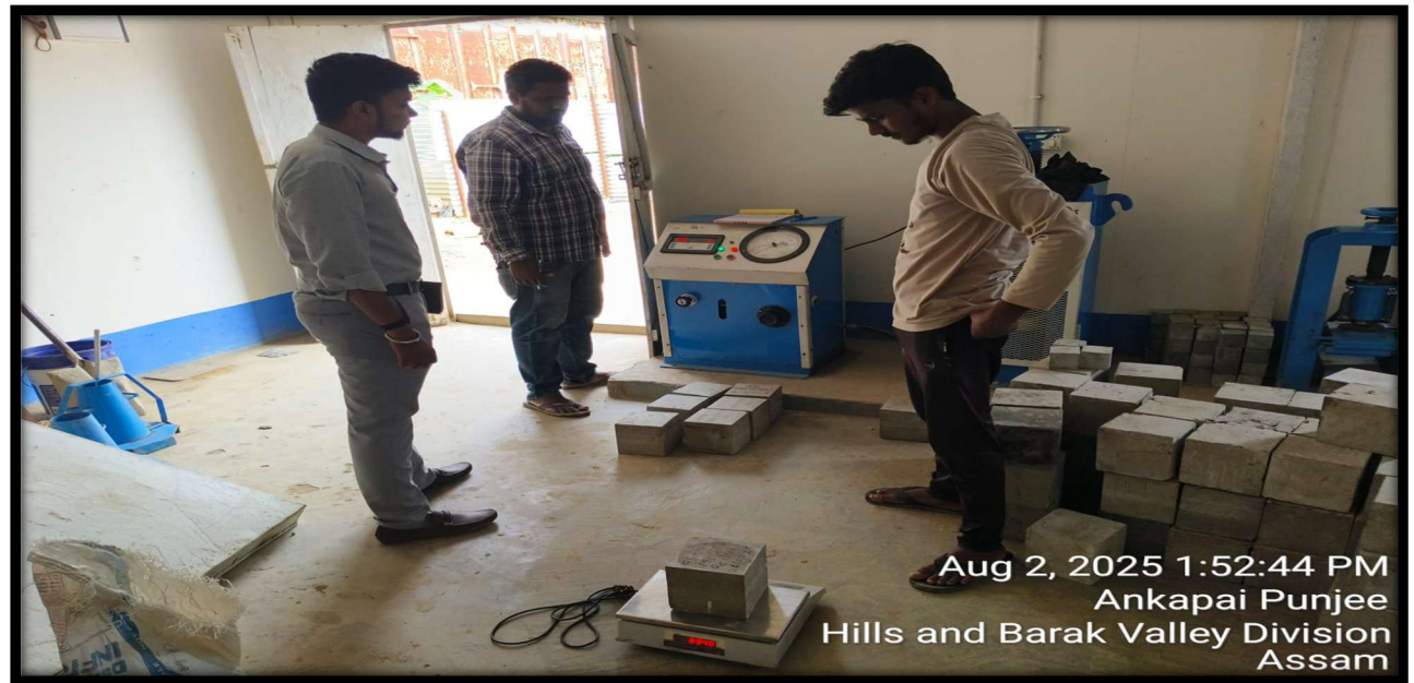
Cube test in presence of IE's representative
