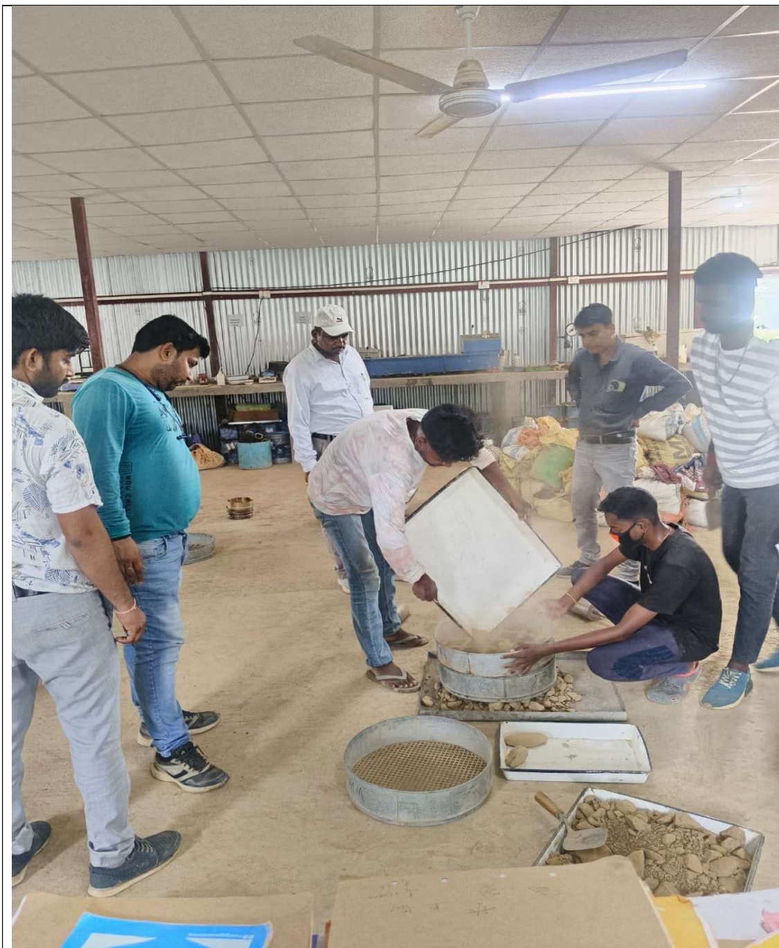
GSB MIX DESIGN CONDUCT WITH IE TEAM AT QA/QC LABORATORY
